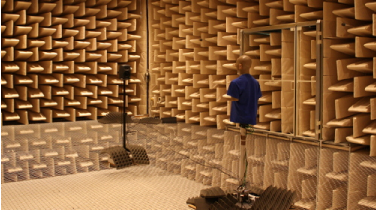
Fig. 7.1: Setup of the KEMAR (Knowles Electronics Manikin for Acoustic Research) and a loudspeaker during a HRTF measurement.
